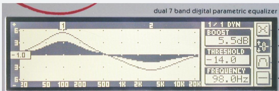
Typical frequency response display with outlined nominal frequency response (thin line, as set by the user) and actual frequency response (solid black) applied by the DSP according to the program level and dynamics parameters.
